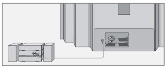
1 Connect the white and red sockets »L R AUDIO OUT« on the television and the corresponding sockets on the HiFi with a cinch cable.
